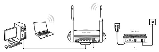
Figure 2-2 Hardware Installation of the TL-WR843ND in Router mode
