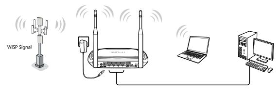
Figure 2-1 Hardware Installation of the TL-WR843ND in WISP Client Router mode
