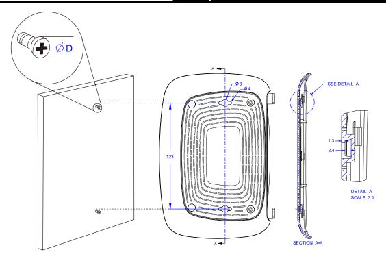
Figure 2-3 Wall-mount Install
