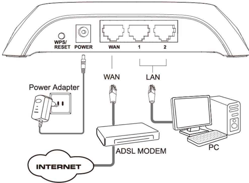
Figure 2-1 Hardware Installation of the 150Mbps Wireless N Router
